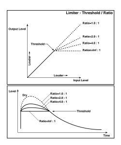
c: Attack d: Release These parameters set the attack time and release time. A higher attack time will cause the compression to be applied more slowly.
